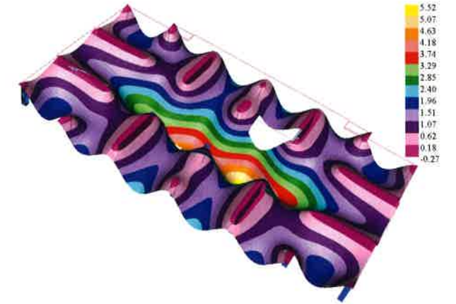
FIGURE 8.5.1-6 Deflected Shape of the Floor System (P118)
